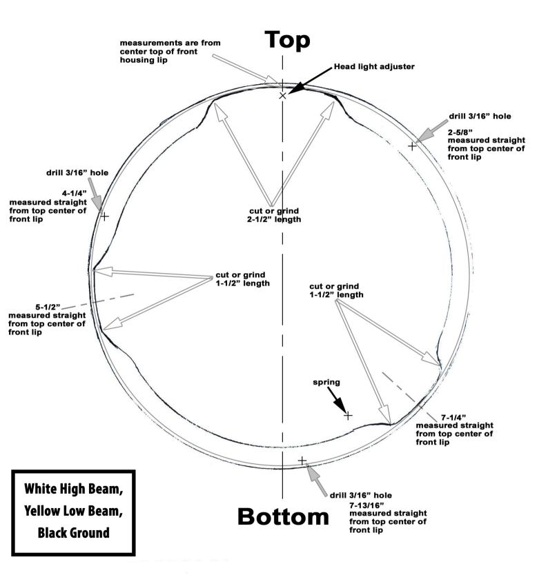
Cut or grind clearances in lip of headlight housing. If ground or cut correctly you can insert the assembled buckets (trim & lens removed) in through the opening. Mark and make sure mounting holes on outer bucket line up with 3 holes and drill in lip of housing.
